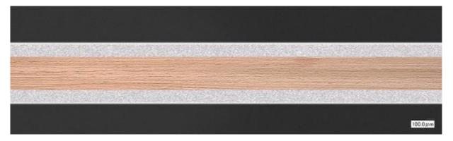
The conductivity is **105.0 IACS%**. The specific gravity is 9.5.
